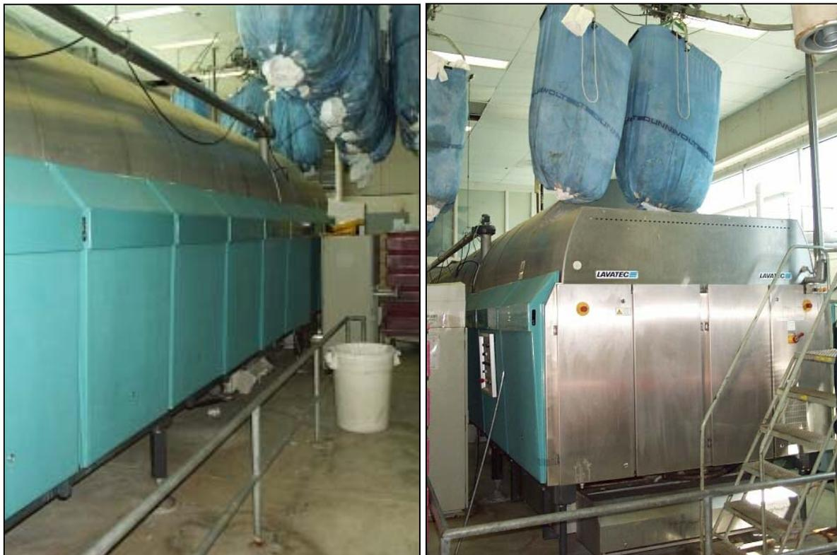
**Figure 3-1 Side (l) and Loading Chute (r) of Lavatec Lavatrac Continuous Batch Washer at NMMC**
